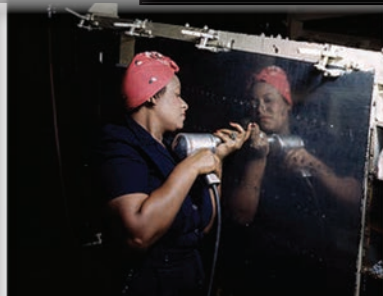
A "Rosie" putting rivets on an Vultee A-31 Vengeance in Nashville, Tennessee in 1943.
